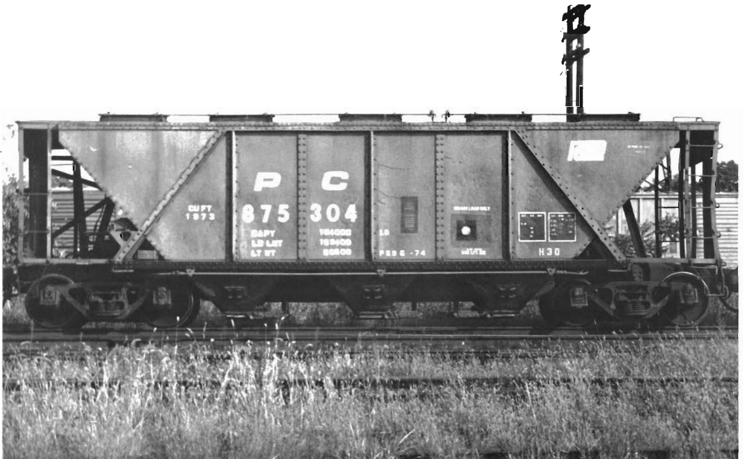
PC 875304 is an old H30 repainted in PC green in 1974. The car's capacity has been increased from the original 70 tons to 77, but this car is stenciled "grain loading only" and it is doubtful that a low-bulk-density item like grain would ever approach this car's weighted capacity. The car is still equipped with friction-bearing trucks, well into the roller-bearing era.
