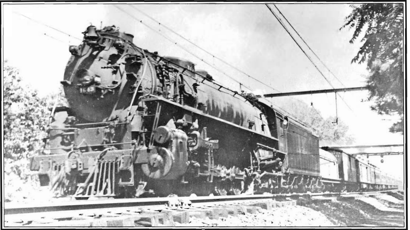
EASTBOUND LACKAWANNA PASSENGER TRAIN at East Orange, New Jersey, on May 26, 1936. The first two cars behind DL&W 4-8-4 No. 1643 were "BFIX" Borden bulk-milk tankcars.
